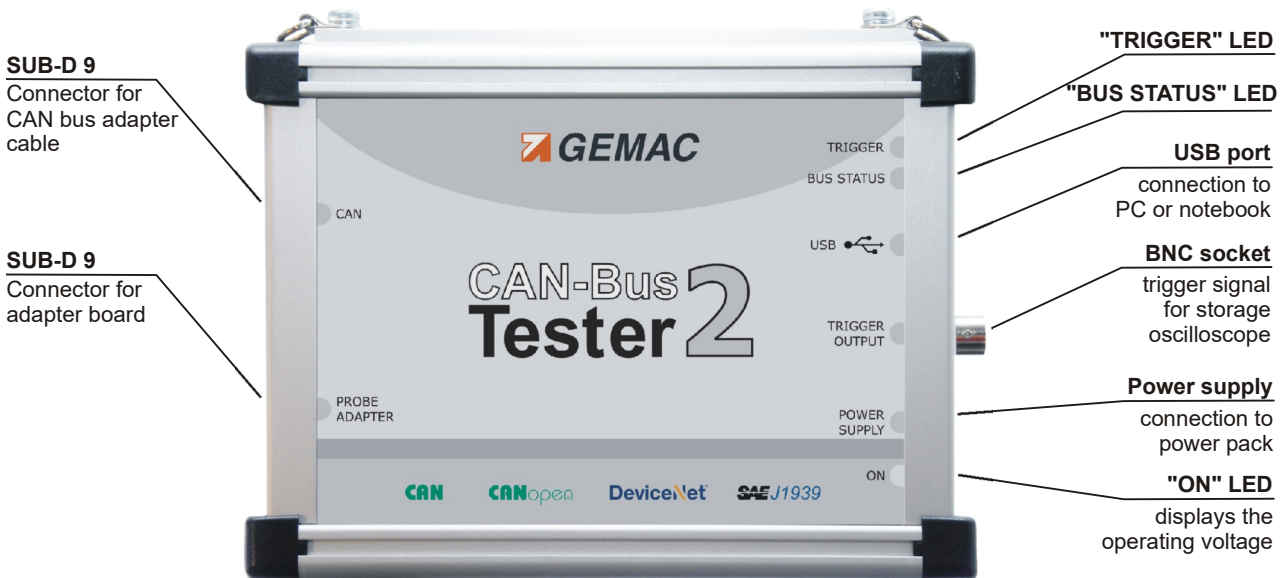
Figure 1: Connections of the CBT2
