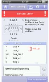
length used. Higher values than expected are an indication of transition resistances in plug and terminal connections.
