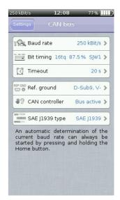
"CAN Level Absolute", as well as to be able to measure the shield voltage, the reference ground against which these levels were measured must be set. Measurement against CAN\_V- (pin 6) of the 9-pin D-Sub CAN socket is set here. If the "CAN\_V-" line is not connected in the connector of the cable you are using, then switch the reference ground to the external ground connection and connect it to the ground of the node to be measured.
