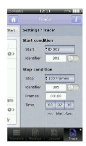
By starting the trace module a new file in the format "can00000.trc" with ascending number is stored in the folder "Tracefiles" on the drive of the CANtouch<sup>®</sup>. The already used space is visualized by means of a progress bar. Upon reaching the reserve capacity (red line), the recording will stop automatically.
