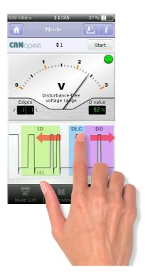
What can I do when  $\stackrel{\bigcirc}{\cup}$  or  $\stackrel{\bigcirc}{\bullet}$  are displayed? Quality value, Disturbance-free voltage range, Edge steepness
