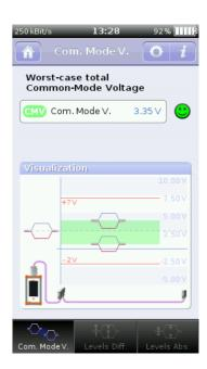
On bus traffic the CANtouch® continuously measures the absolute signal levels of all CAN modules relative to the position of the tester and determines highest difference of their signal levels – the worst-case total common-mode voltage.
